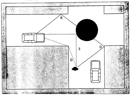
Scattering, which follows the same physical principles as diffraction, causes energy from a transmitter to be reradiated in many different directions. It is the most difficult mechanism to predict.
