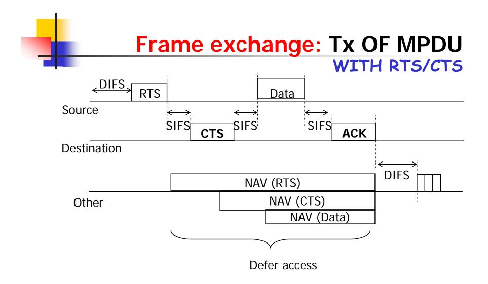
NAV: network allocation vector indicates the time amount that must elapse until the current Tx is complete and the channel can be sample again for idle status
